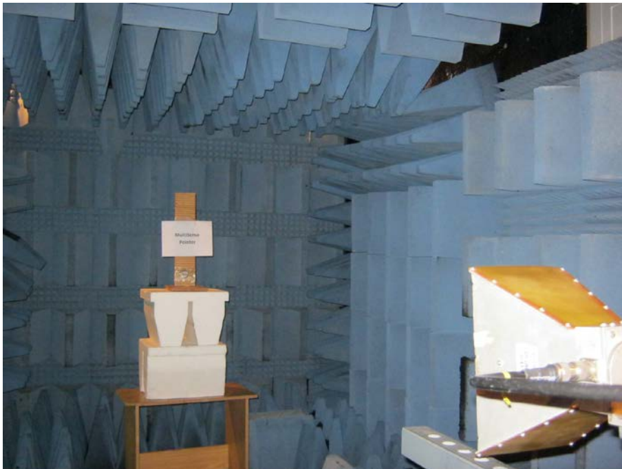
Figure 15 Spurious Emission (Tx/Rx) Test
